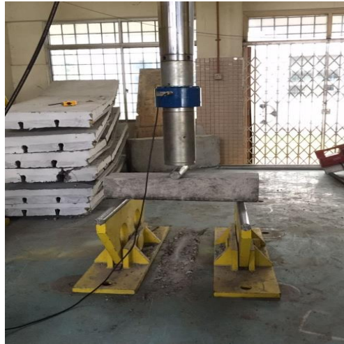
FIGURE 12. Determination of flexural strength
