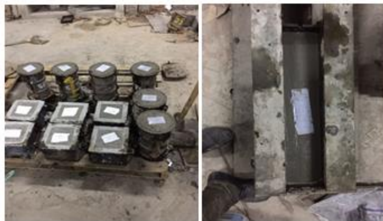
FIGURE 5. Casting of cubes, cylinder and beams
